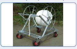
A heavy duty galvanised steel trolley with a central "bobbin" which holds two 220-metre boundary ropes. A handle winds the rope onto the bobbin. Size: 1070mm wide x 1270mm long x 1350mm high.
