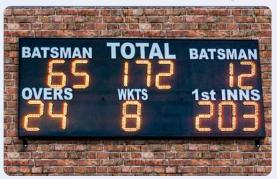
This 15 digit scoreboard is designed to be a versatile scoreboard that can be easily fitted to the outside of a pavilion, while being light enough to be removed. The scoreboard uses 250mm amber LED digits which create a bright and clear number. The Club Scoreboards displays, Both Batting Scores, Overs, Wickets, 1s Innings and the Total Score.
