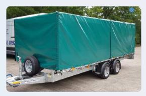
We can produce trailer covers to suit any size from a standard boxed to bespoke to pick up. All of our covers are made to measure and produced to the highest specification. Our waterproof trailer covers are competitively priced and made from a minimum weight of 580gsm to a maximum of 900gsm PVC.
